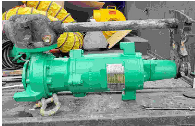
New lift station pumps.
