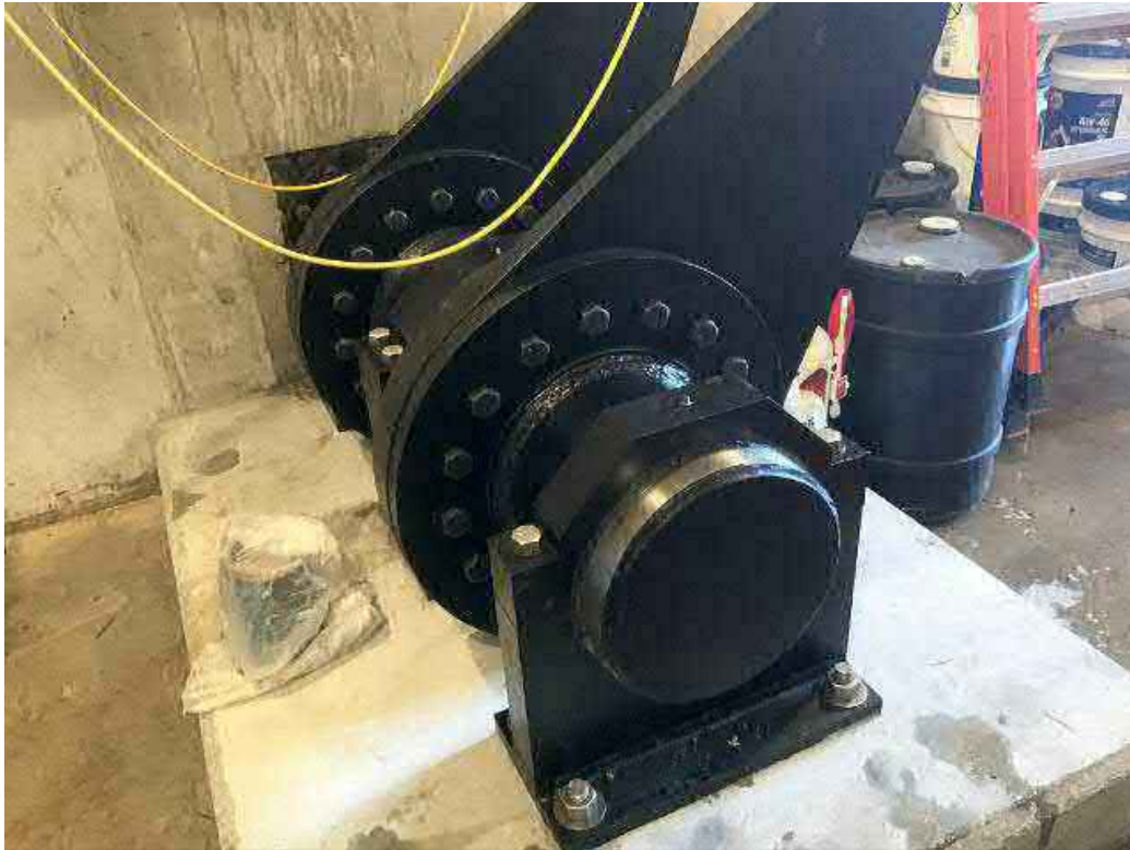
Torque arm - bearings and bearing mounts.
