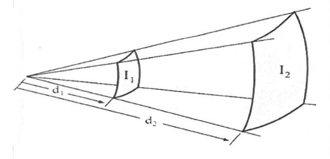
The Inverse Square Law gives us a logical first estimate for the intensity of sound as it travels over a distance. If we know the Intensity 1 (i1) at a given Distance 1 (d1) then we can calculate the Intensity 2 (i2) at a given Distance 2 (d2).
