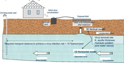
Septic systems are underground wastewater treatment structures, commonly used in rural areas without centralized sewer systems. They use a combination of nature and proven technology to treat wastewater from household plumbing produced by bathrooms, kitchen drains, and laundry.
